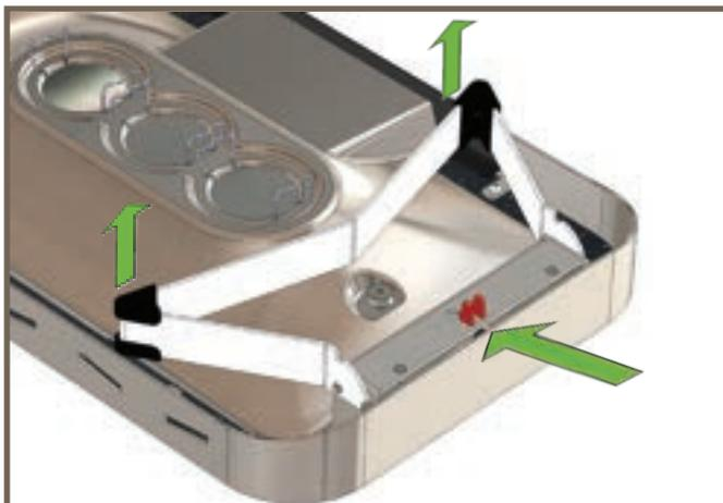
2. To unfold the legs, firstly move and hold the locking levers (1) in the direction shown by the arrow cut-outs. Then fold the legs (2) to the upright position in the direction of the green arrows.
