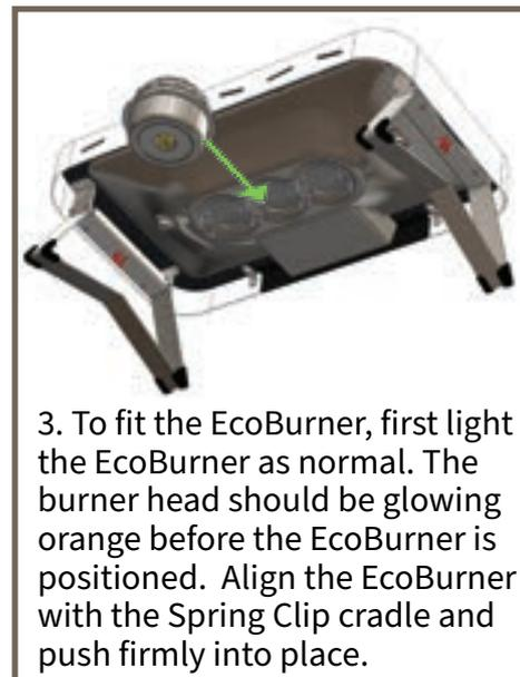
3. To fit the EcoBurner, first light the EcoBurner as normal. The burner head should be glowing orange before the EcoBurner is positioned. Align the EcoBurner with the Spring Clip cradle and push firmly into place.
